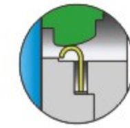
1. Three eccentric metal seal
