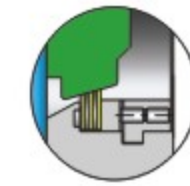
2. Eccentric three-layer composite metal sealing
