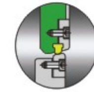
6. The rubber seal (which can replace the valve seat)
